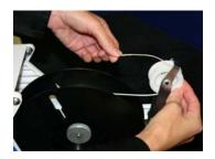
3) Feed tie material under small roller on brake arm, then over top of roller and pull towards machine.
