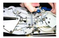
6) Continue slowly inserting the ribbon into Pinion Support Channel until the ribbon appears just beyond the cutter. Make sure that the ribbon is under the lip of the white plastic ribbon guide.
