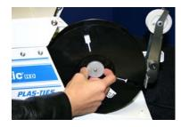
2) Place spool on spindle and tighten Knurled Nut snugly onto the spindle to secure spool.
