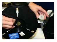
1) Unscrew Knurled Nut, then place spool of tie material in right hand with label facing palm.
