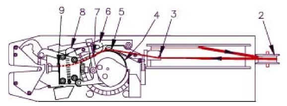
Note: Make sure material is straight or curved slightly towards machine (11) when inserted into Pinion Support Channel (7), not kinked or curved as per (10).
